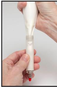
Place a storage cap (D) onto the end of cartridge (A) to retain contents. Pipe contents into cartridge to about 2/3 full. Insert a 'follower' (B), solid end first, into cartridge. Use the puller tool (H) to gently compress contents into the cartridge.
